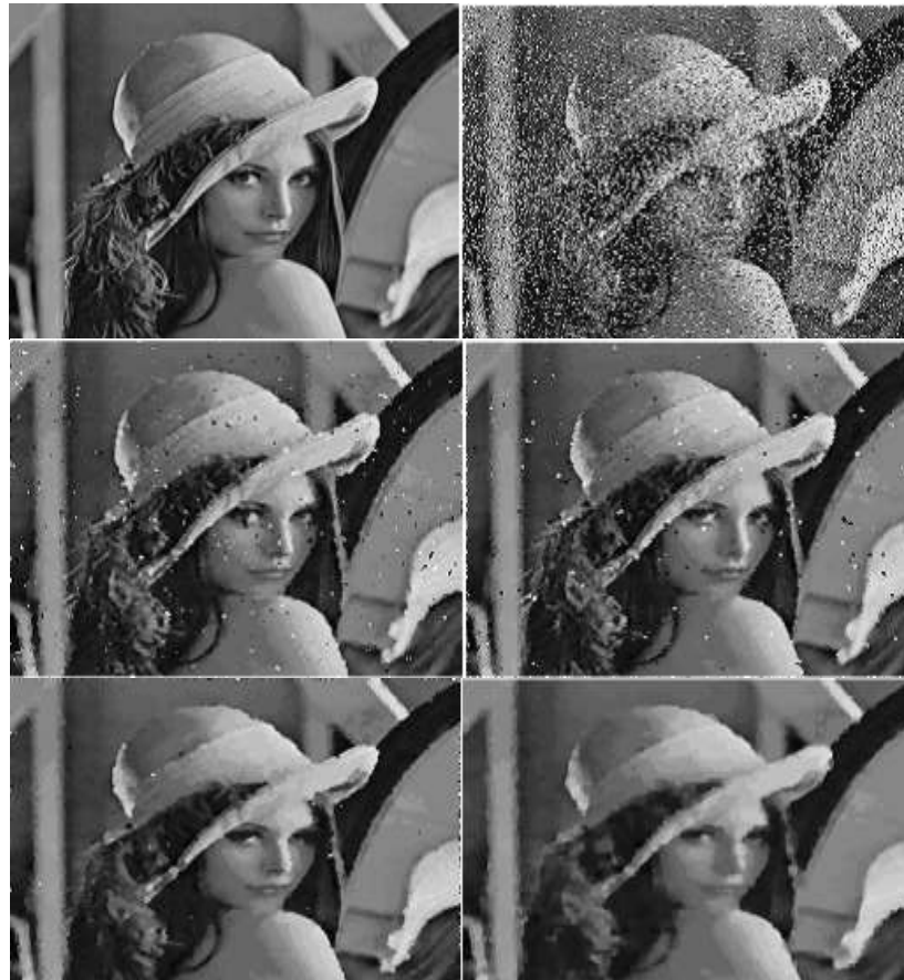
Fig.3.1. simulation result for lenna image:(a)original image (b) corrupted with 30% noise (c)output from median filter (d)output from cwm filter(e)output from pwmad filter(f) output from ocs filter
