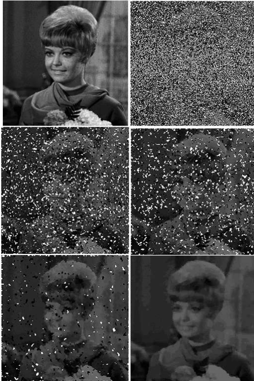
Fig.3.4. simulation result for girl image: (a)original image (b) corrupted with 60% noise (c)output from median filter (d)output from cwm filter (e)output from pwmad filter (f) output from ocs filter
