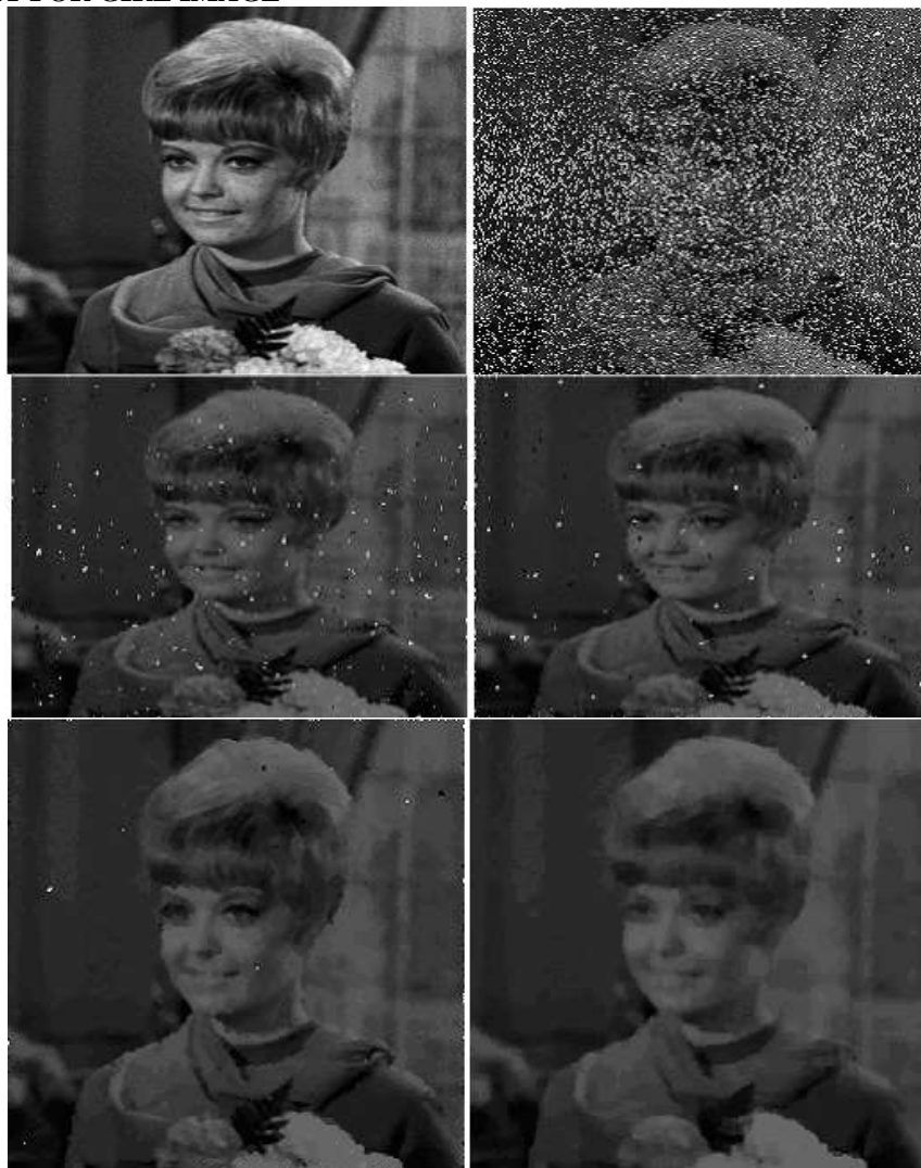
Fig.3.3. simulation result for girl image: (a)original image (b) corrupted with 30% noise (c)output from median filter (d)output from cwm filter (e)output from pwmad filter (f) output from ocs filter
